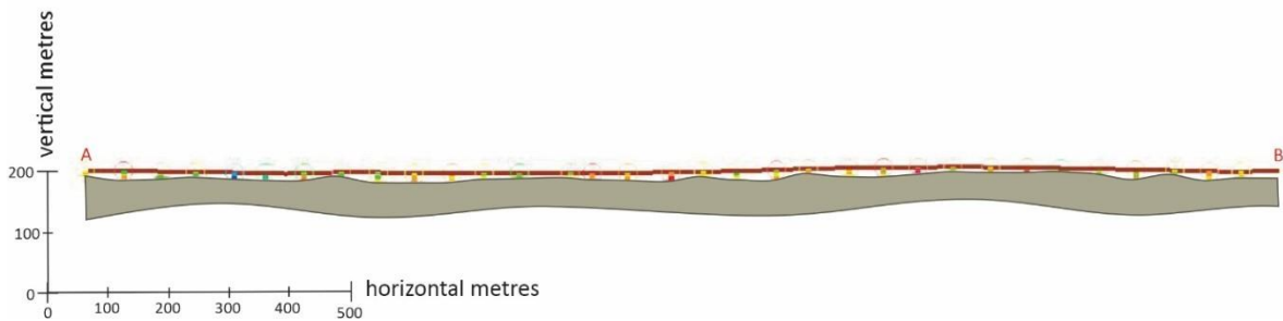
Figure 2: Sandy Mitchell Project west to east cross section at 8193750 m north through the REE & HM sand, showing drill data from the Stage 1 resource AC drill grid coloured for monazite equivalent.
