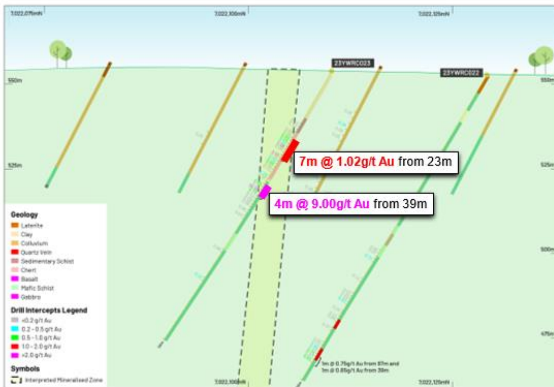
Figure 2: Cross section at Barwidgee Fault Prospect drilling.
