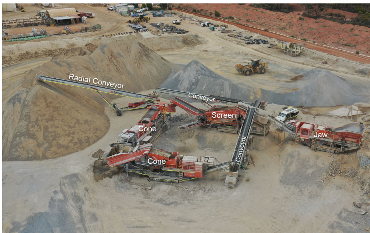
Figure 2: Beacon Crushing Circuit on Jaurdi ROM
