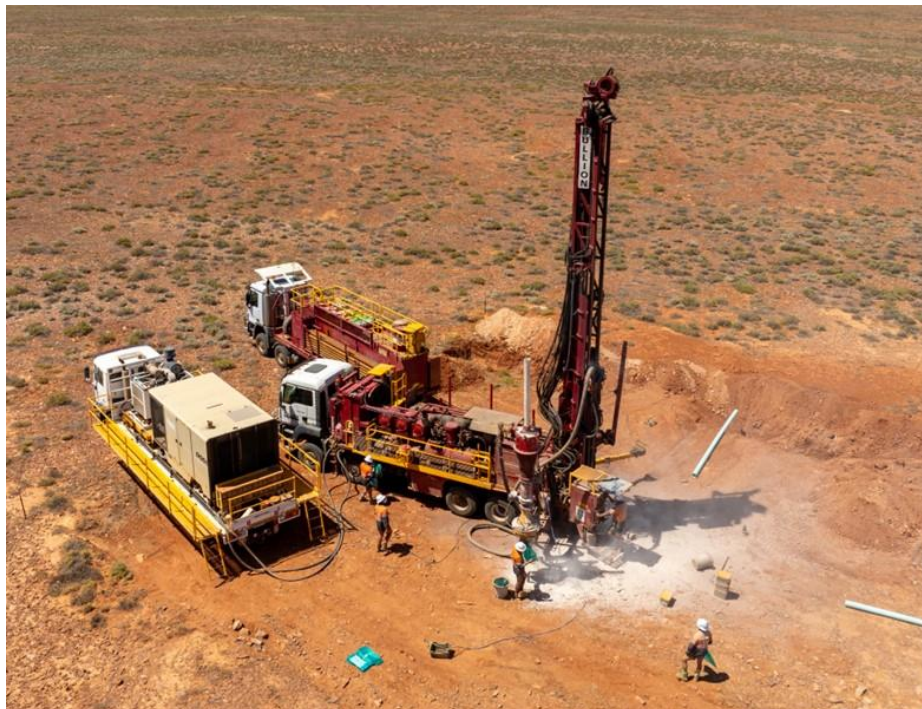
Figure 1 RC drill rig commencing operations at Emmie Bluff
