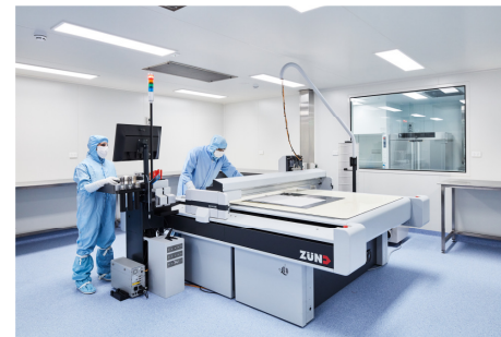
Inside new cleanroom facility: shape cutting and ultrasonic welding table- Hernia
