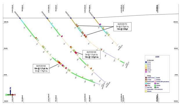
Figure 6: BARC00164, 169 and 172 cross sections
