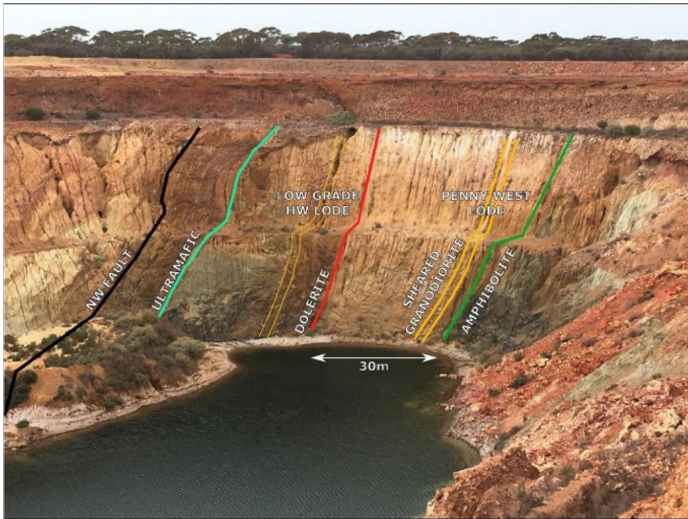
South wall (looking South towards Strata's Penny South Project) of the Penny West pit showing stratigraphic relationships to the Penny West Lode, noting high-grade (FW) and lower-grade lode (HW)
