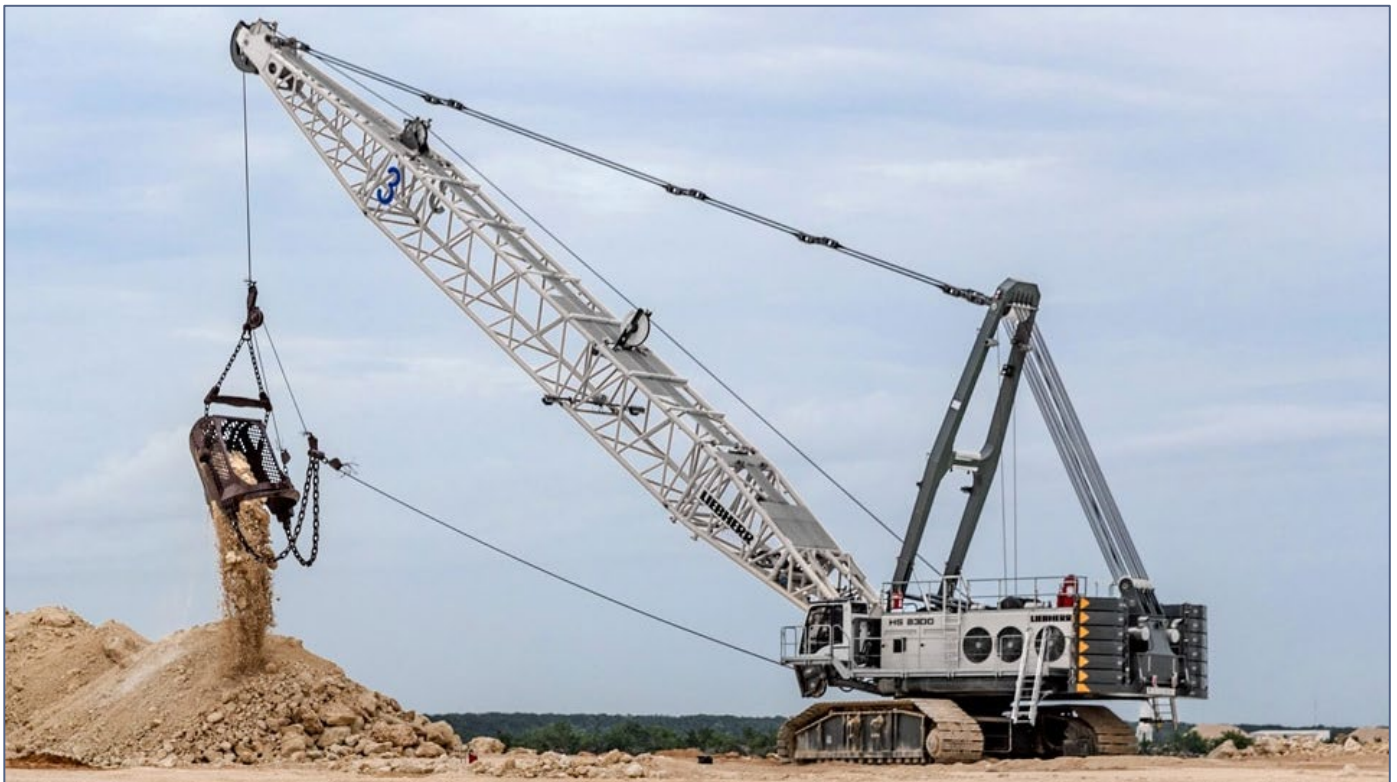
Figure 10: Example of a dragline excavator in action (Source: Liebherr Group)
