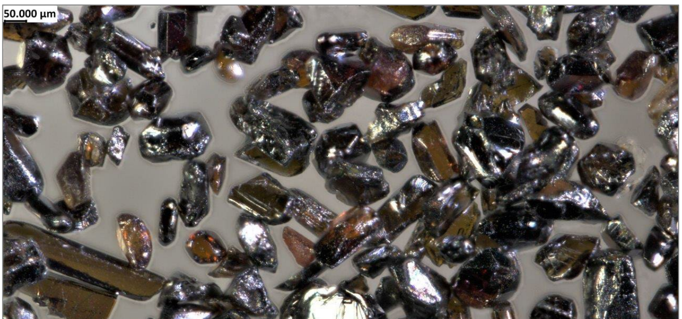
Figure 17: Photomicrograph of high-purity rutile product
